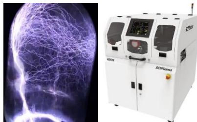
Figure 2: (a) The formation of an Argon plasma [3] (b) Industrial semiconductor manufacturing plasma system [4].
