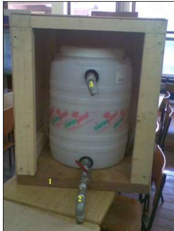
Figure 2. Storage tank – plastic barrel of 60 litres capacity – in the box prior to thermal insulation. 1 – 5 cm thick plank, 2 – discharge pipe, 3 – overflow valve
