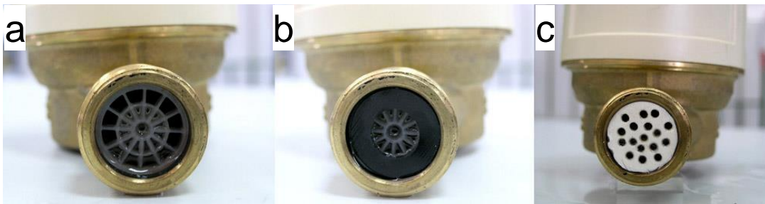
Figure 6. Partial blockage of the inlet strainer of a single jet meter
