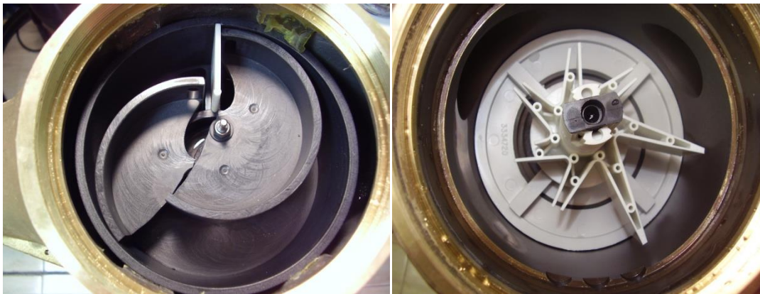
Figure 2. Examples of broken mechanical meters because of high flows
